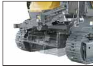
Conveyor elevation system
