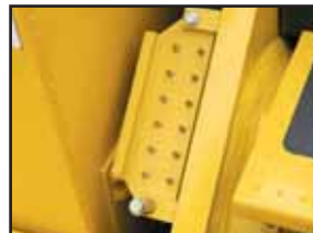
Centralised greasing system
