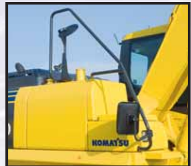
Large handrail for safe access
