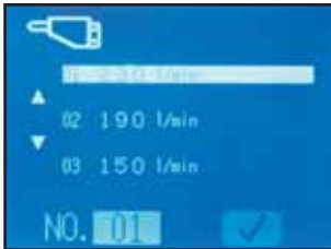
Hydraulic flow general adjustment screen in B (breaker) mode
