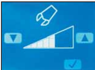
Fine tune hydraulic flow adjustment screen in P (power) or E (economy) mode
