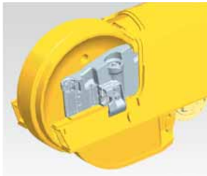
Self-adjusting idler support
