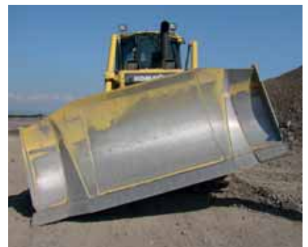
Hydraulically adjustable tilt: 870 mm
