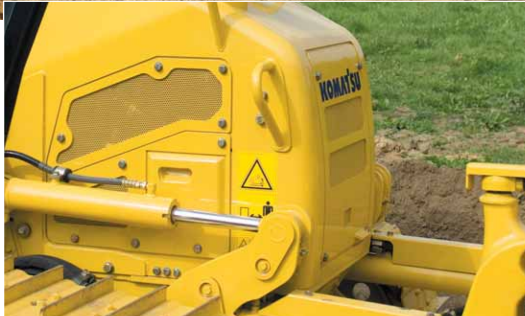
One-piece nose guard Simplified high-rigidity structure with thick plates reduces vibration and increases the lifetime.
